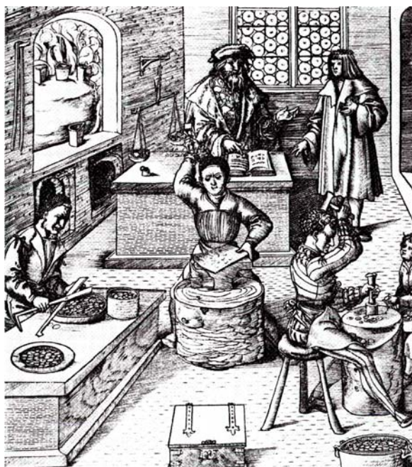
Figure 3.2 Medieval woodcut illustrating a mint worker striking coins using a hammer. 3 Note that the man on the right of the picture uses a lower (obverse) die secured in a sturdy log to form his work station whilst he secures the upper (reverse) die in place with his left hand as he strikes it with a hammer.
